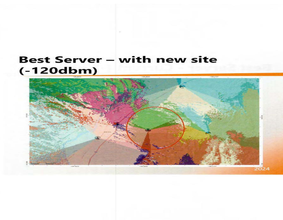
Figure 7. Biwabkos slide 16 — "Best Server — Proposed." The colored zone corresponding to the proposed site is the geographic region in which the new RAD center is the strongest server (dominant new server lobe). The lobe is concentrated to the south, southwest, and west of the proposed-site marker, extending toward the Bernalillo basin and the Sandia foothills, and overlapping substantially with sectors already served by existing corridor towers.
