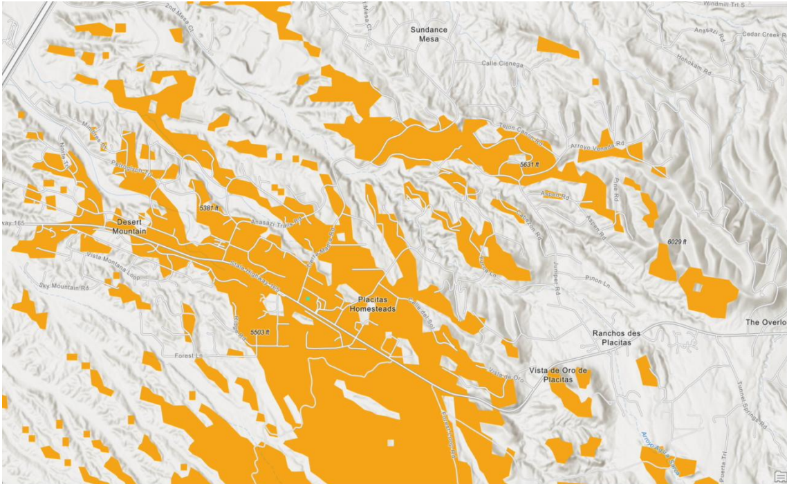
Figure 1. ArcGIS Pro geometric viewshed analysis for the proposed 75-ft monopole at 221 NM-165 (green dot at the labeled "5503 ft" elevation marker), J. Branum, March 2026. Orange shading indicates terrain at 5 ft AGL that has geometric line of sight to the antenna top. Unshaded (white) terrain is in geometric shadow. The eastern portion of the map — including Sundance Mesa, Ranchos des Placitas, Vista de Oro, the upper Las Huertas drainage approaching The Overlook, and the eastern arroyo system — is overwhelmingly unshaded, indicating geometric shadow.
