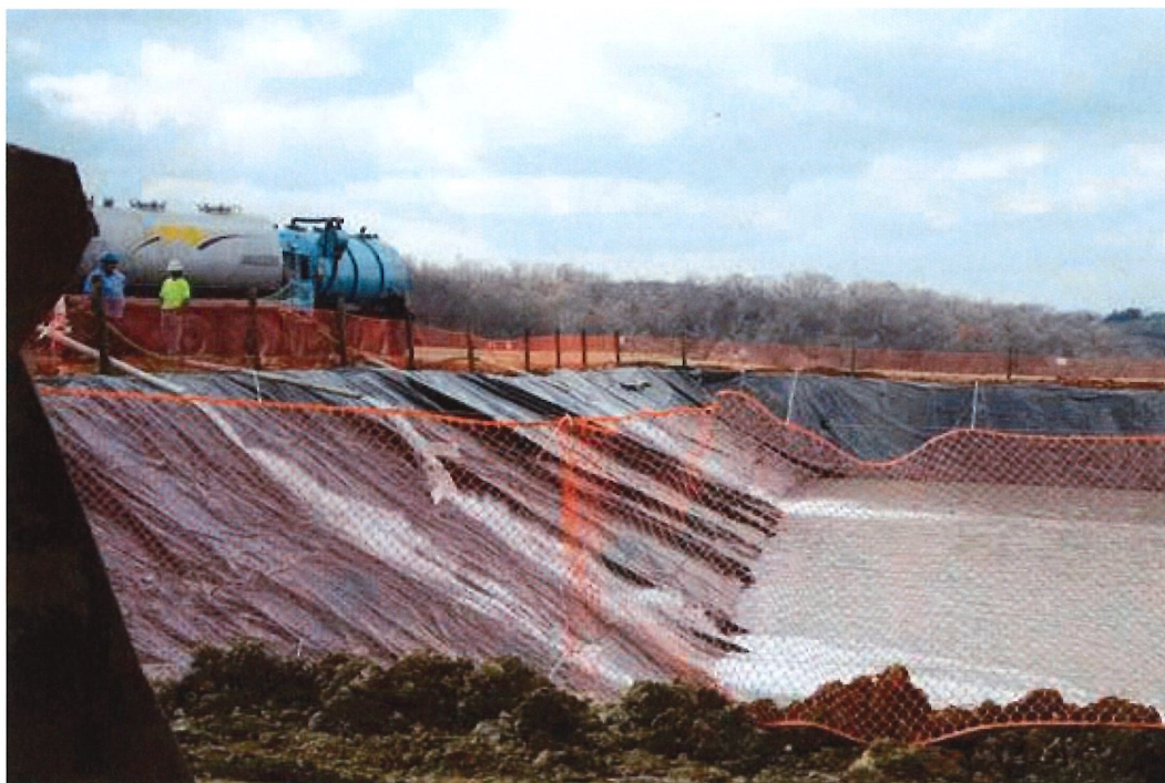
The disposal of fracking wastewater in open pits contributes to air pollution, while leakage from improperly lined pits has contaminated groundwater and surface water. Chemicals present in fracking wastewater have been linked to serious health problems, including cancer. Credit: Mark Schmerling
