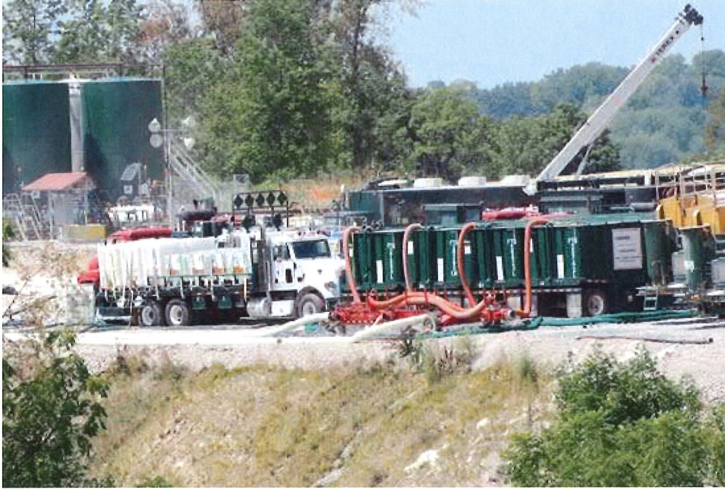
Fracking requires millions of gallons of water and large quantities of sand and chemicals, all of which must be transported to well sites, inflicting damage on local roads. Above, a well site in Washington County, Pa. Credit: Robert Donnan
