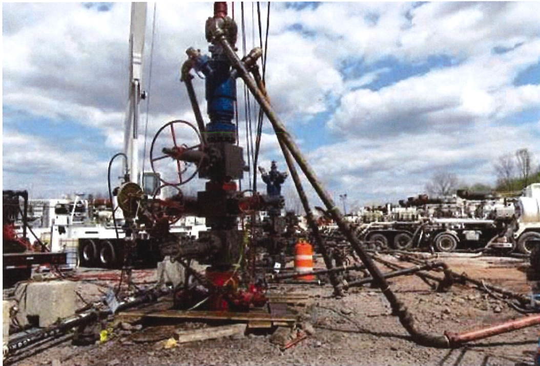
Equipment is put in place in preparation for hydraulic fracturing at a well site in Troy, Pa. In hydraulic fracturing, a combination of water, sand and chemicals is injected at high pressure to fracture oil or gas-bearing rock formations deep underground. Credit: New York Department of Environmental Conservation
